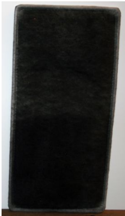
MVHR filter after 6 months in Central London Image from bere:architects.co.uk
